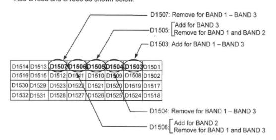
Depending on the version of the transceiver you have, some diodes maybe already installed or missing.
