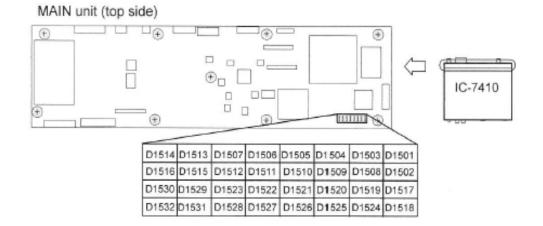
TX frequency coverage expansion (HF/50MHz bands)
