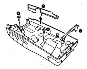
Push the cross key section (a) on the key top upward from the front with a finger. The control PC board is lifted and removed from the case.
