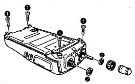
Pull out the panel assembly (3) and separate the chassis from the case gradually, beginning with the bottom (4).
