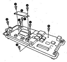
Finally, remove the solder ( ) from the ANT terminal to remove the RF PC board from the chassis. Take care not to drop and lose the battery terminal ( ) on the chassis.
