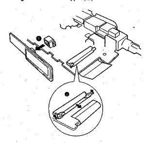
Release the four hooks (\*) on the right guide from the control PC board. The right guide and LCD assembly (\*) will be detached.
