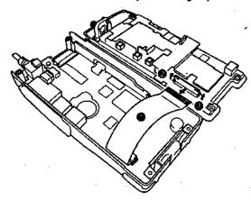
To remove the control PC board, remove the holder (3) and the two screws (3) holding the PC board.
